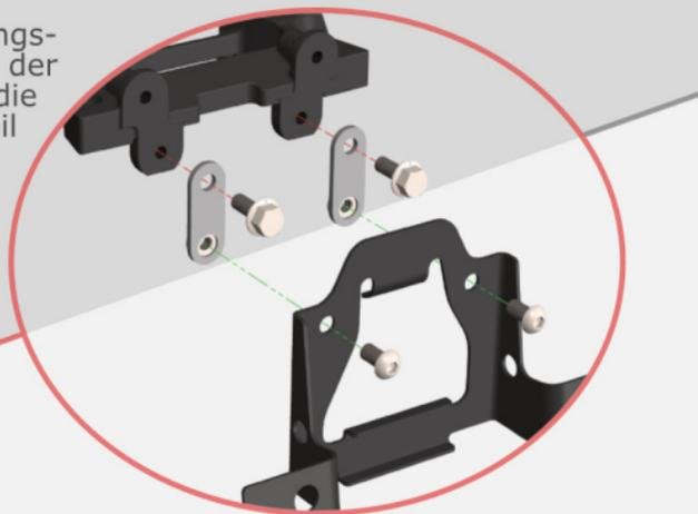
*The holder for windshield mount is a connecting piece for mounting the windshield mount when using the VMT handlebar riser **S25Z**. First remove the fairing washer and then mount the component as shown in this graphic.*
